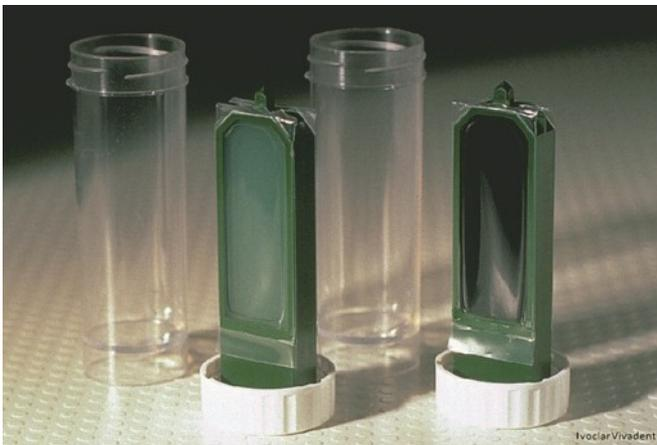
**Fig. 12** "Double dip" for the detection of SM and LB, Rogosa agar (light side) and SM-modified MSB agar (dark side, fig. courtesy of Ivoclar Vivadent, Ellwangen).
